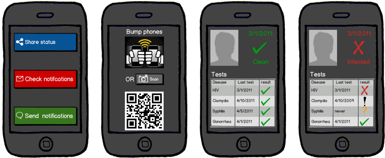
Figure 3: A UI mockup for TruSTI. From the left: a Prover selects “Share” on the home screen; the parties bump their phones or scan a QR code to handshake; the Prover’s STI results are displayed on the Verifying user’s smartphone. The Verifier must inspect the prover’s photograph manually. This is executed symmetrically to exchange STI results.
