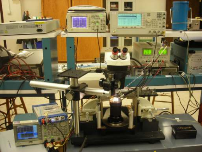
Fig. 5. CRP Collection from ASIC Arbiter PUFs
